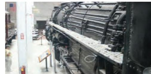
Side view of the Big Boy. With its tender attached, the unit is bigger than any train engine to ever run on US rails. Its wheel configuration is 4-8-8-4-2.
